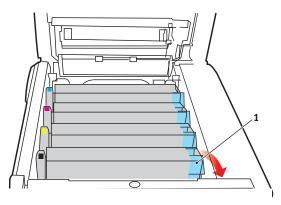
**3.** Lift the right-hand end of the cartridge and then draw the cartridge to the right to release the left-hand end as shown, and withdraw the toner cartridge and image drum unit together out of the printer.
